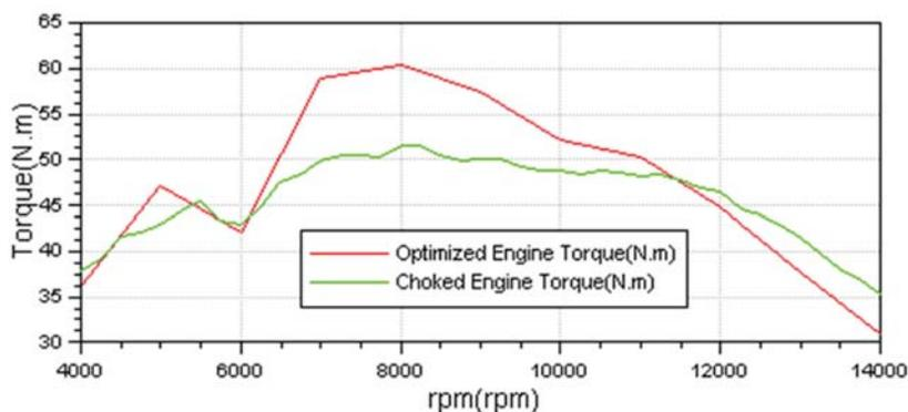
Fig. 3 - Engine performance after the optimization process
